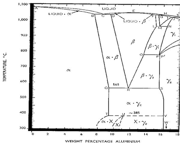
Figure 1: Cu-Al phase diagram. (Source: Copper Development Association. (1992). Equilibrium Diagrams. CDA Publication No.94, p. 17.)
